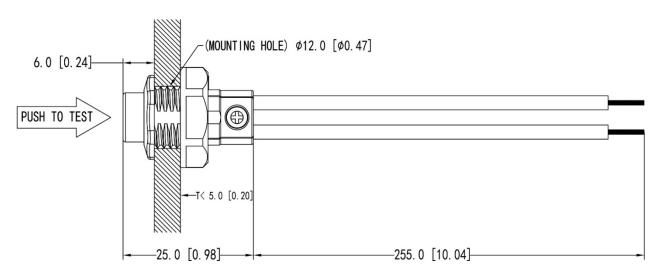
Dimension unit: mm [inch] / Tolerance: ±1[0.04]
